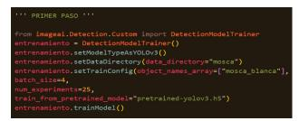
For the creation of a model, the classes are required in relation to the images that were labeled, then yolov3 is taken as a pre-training model. Finally, the Create\_Model.py file was executed, where an optimal model for pest detection was obtained.
