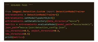
In order to select an accurate detection model, it is necessary to evaluate it based on the config.json file that stores the detection configuration after having trained the set of labeled images. Model Testing
