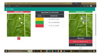
After processing the image, the analysis interface is presented, where the percentage of affectation is shown, which allows it to be classified between one of the three affectation indicators (there is no pest when it is 0%, moderate when it is between 1-69% and serious between 70-100%). These values are generated from the execution of three Deep Learning algorithms that allowed the labeling, training, and validation of objects in images.
