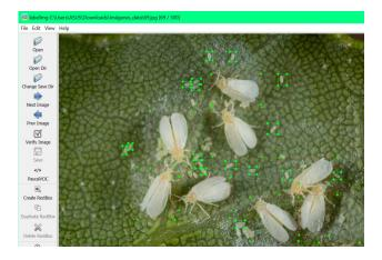
To start the detection, the insects (objects) within the images had to be previously labeled, in this first version the whitefly, for the labeling the free use tool labelImg was used, which allows the dimensions of the insects to be stored in XML files. that were captured in the images.
